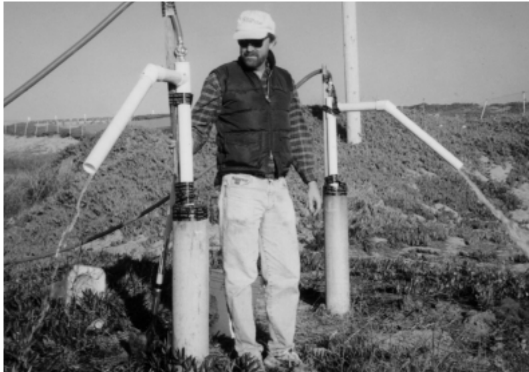
Tom Lindberg, MPWMD, pumping water prior to water quality sample collection from wells that are part of the District's Seaside Basin coastal monitor well network.
