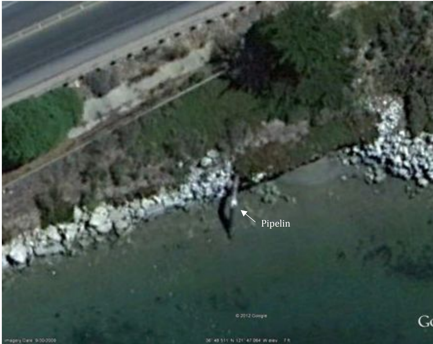
Figure 4. Photograph of the abandoned fuel oil pipeline where it can first be seen on shore, south of the Highway 1 bridge and just north of the Moss Landing Power Plant.
